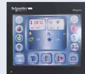
Touch screen control panel with PLC. Panel de control con pantalla digital PLC.
